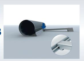
Attach the stabilizing foot to the lower panel profile.
