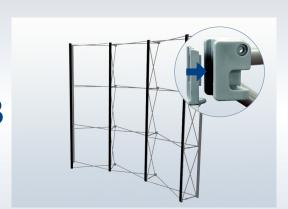
Click the magnetic bar into the hubs of the system. Repeat until all the magnetic bars are in place.
